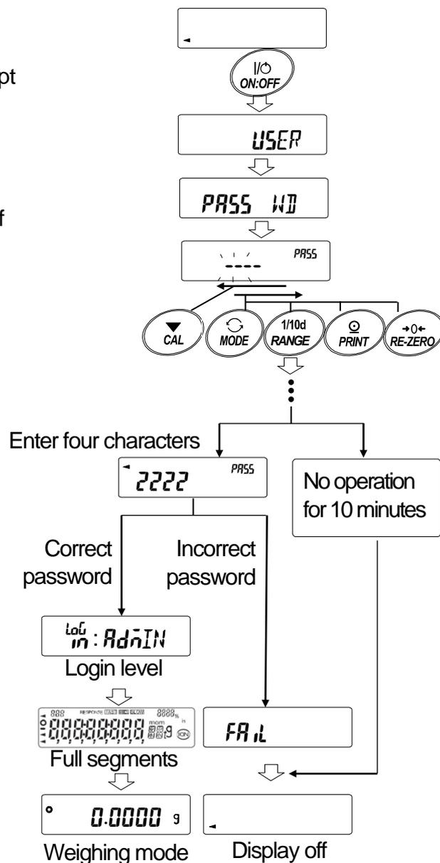
**Note** When the balance software version is 1.50 to 1.64, the login level is not displayed when logged in.
