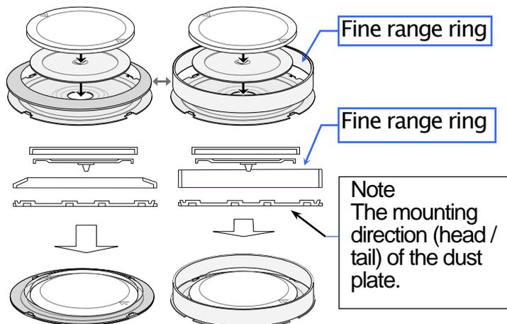
Use the fine range ring in place of the breeze break ring to avoid errors caused by drafts when weighing with a readability of 0.01 mg.
