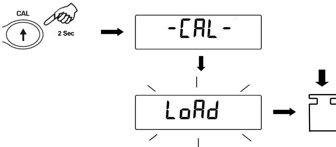
2. Load on the pan a weight equal higher or lower than default calibration weight; the balance will recognize it as valid weight if equal or higher than calibration weight as long as it is a whole number in comparison with the most meaningful digit of calibration weight .
