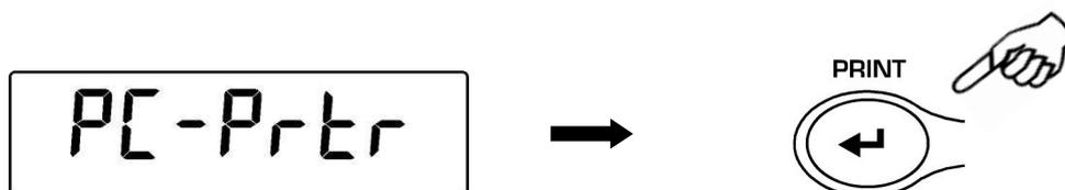
2. Press the **MENU** button until the “**PC cont**” is displayed to choose continuous print or “**PC CMd**” to choose print to PC at user command, then press the **PRINT** button to confirm the choice.
