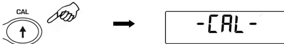
2. When calibration weight value starts to flash, load the weight on the pan.
