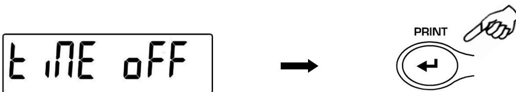
2. Pressing **MENU** or **CAL** button it will be possible to scroll forward or backward the different auto power-off modes, select the one you wish and then confirm it by pressing the **PRINT** button
