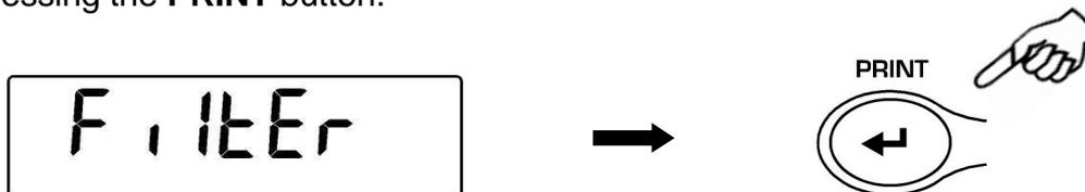
2. Pressing **MENU** or **CAL** button it will be possible to scroll forward or backward the different filtering levels, select the one you wish and then confirm it by pressing the **PRINT** button
