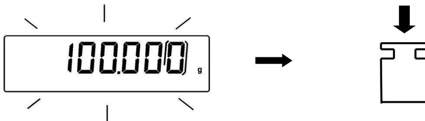
3. The display will stop flashing, indicating calibration weight value. Once the calibration is effected will be shown the value of the calibrated weight and the current unit of measure.
