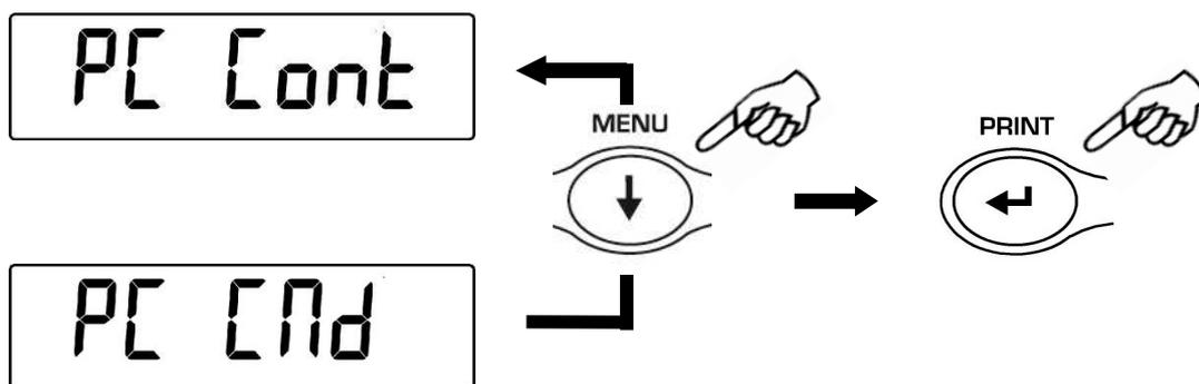
3. After having selected the desired transmission mode, press the **MENU** button to go to next parameter or the **CAL** button to go to previous.
