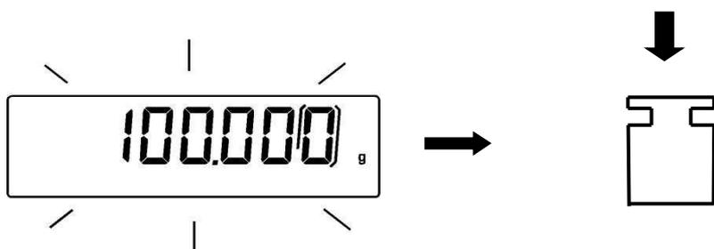
3. Wait the acoustic alarm and that the displayed calibrated weight value stops flashing, then unload the weight from balance pan.
