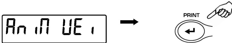
2. Set the desired period time from 5 to 90 sec. using the button **MENU** to decrement and **CAL** to increment time. Confirm by pressing the **PRINT** button.
