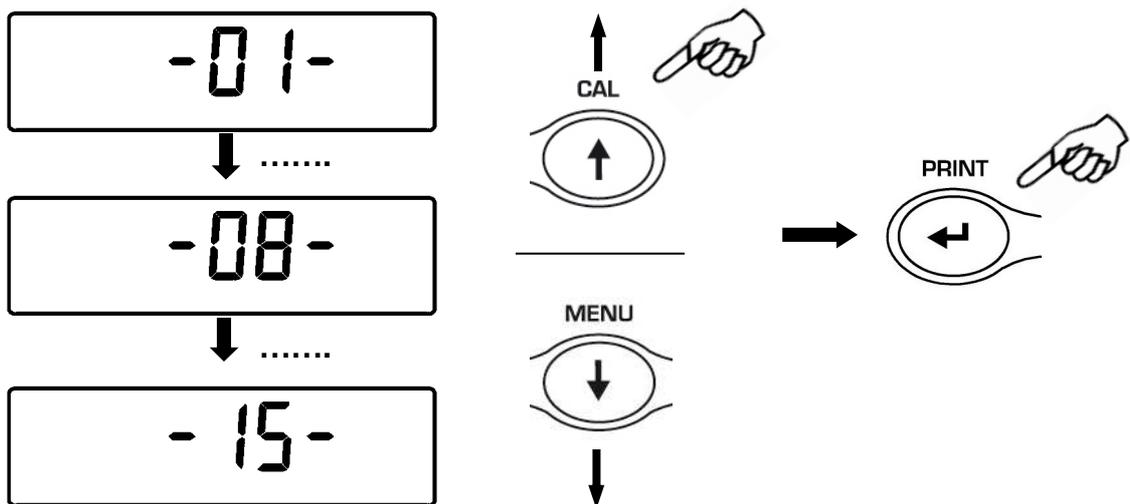
3. After you have confirmed the contrast level desired, press the **MENU** button to go to the next parameter or the **CAL** button to go to previous one.
