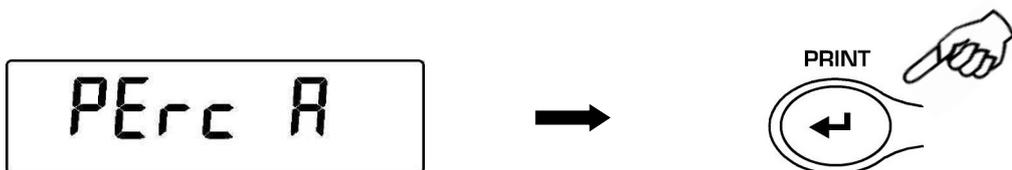
3. Tare function will be performed and will be shown on the display the string **"Load"**. Then load on the weighing pan the reference and press the **PRINT** button, the string **"Load"** will start to flash and once the weight is acquired will be visualized the value with the % indication.
