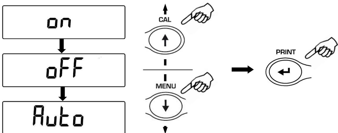
3. After having selected the backlight working mode you wish, press the **MENU** button to go to next parameter or the **CAL** button to go to previous one.
