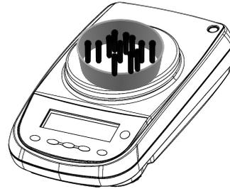
As soon as it is reached a sufficient number of pieces, this number is displayed and it will be possible to go on with count by loading the pieces count on the balance pan.
