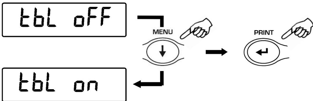
3. After you have chosen the mode “TBL ON” the balance will automatically restart and the message “TABLET” will appear on the display of balance. From this moment the interface device with the balance is the tablet.
