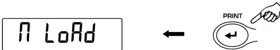
2. Activation of this function is indicated by the visualization of the letter **M** on the last digit on the display.
