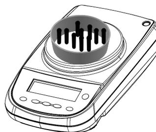
If the number of samples is enough (for example 10 as in figure), then this number will be displayed and it will be possible to go on by loading the pieces to count on the balance pan.
