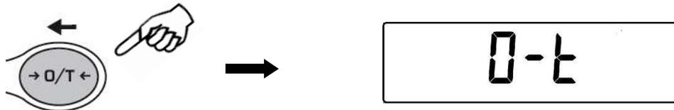
3. After reaching stability, the value "0.000" will be displayed. If the stability is not reached (due to air flows or vibrations or other disturbs) the dashes will remain displayed.
