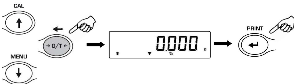
4. Press **PRINT** button when the desired value of the reference weight is inserted
