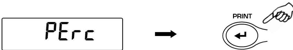
2. Press the MENU button to select the **"Perc A"** function and press **PRINT** button to confirm.
