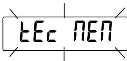
5. After having stored the value of internal calibration weight, balance returns to normal weighing conditions.
