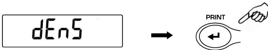
2. Using the **MENU** button, select the function “d Liquid” and confirm this with **PRINT**
