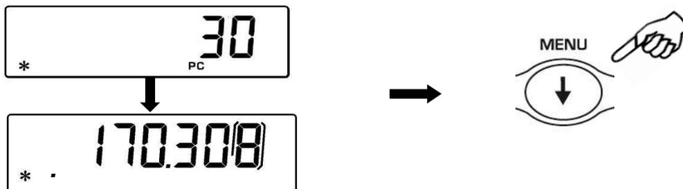
2. In order to display the weight of single piece from the total number of pieces press and keep pressed the **MENU** button until the acoustic alarm gets mute.
