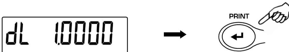
4. It is possible to set a different value using the **CAL** e **MENU** buttons for increase and decrease the value and using the **O/T** button for skip to the others digits. Keeping presses the O/T button is possible to delete the inserted value.
