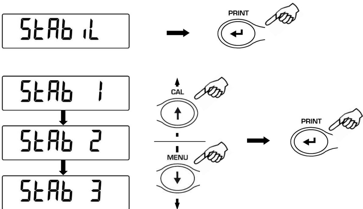
3. After having selected the stability level you wish, press the **MENU** button to go to next parameter or the **CAL** button to go to previous one.
