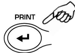
2. Select serial data transmission speed (1200-2400-4800-9600 baud). Pressing **MENU** or **CAL** buttons it will be possible to scroll forward or backward through the different transmission speeds, then confirm your choice by pressing **PRINT** button.
