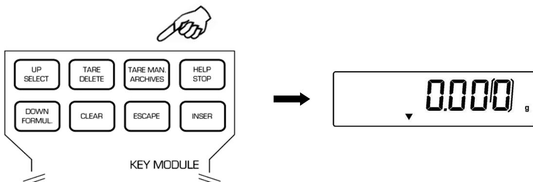
2. Press **CLEAR** to set at zero the previous value (if any) then insert the new value using the alphanumeric buttons placed on the bottom part of alphanumeric keyboard.
