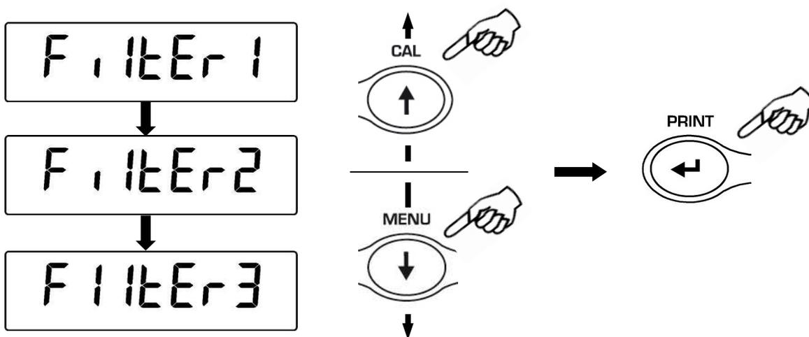
3. After having selected the filtering level you wish, press the **MENU** button to go to next parameter or **CAL** to go to previous one.
