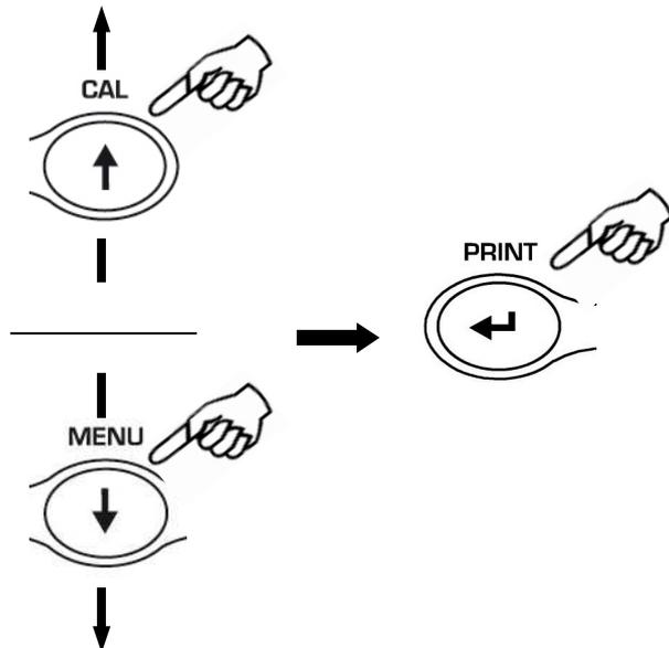
3. After having selected the transmission speed you wish, press the **MENU** button to go to next parameter or **CAL** button to go to previous one.
